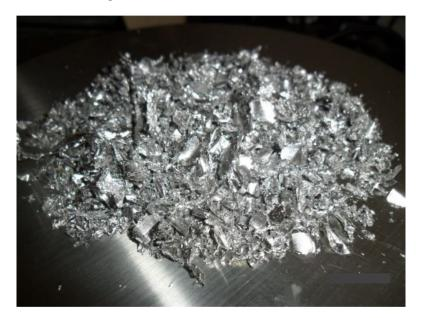
Figure 10 - Recovered solder of PS-PCB
