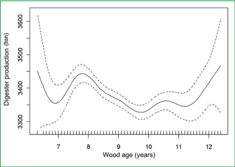
Figure 5 – Smoothed curve of digester production as a function of wood age (Source: the authors)
