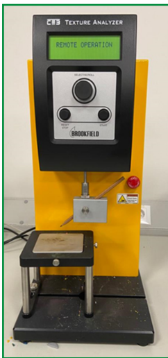
Figure 4 – Point (graphite) breaking test machine setup
