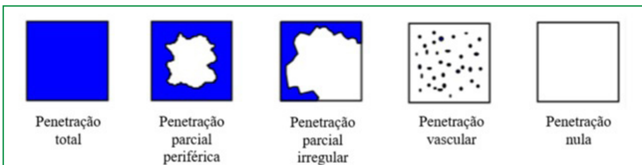
Figure 2 – Classification of specimens according to treatment penetration
