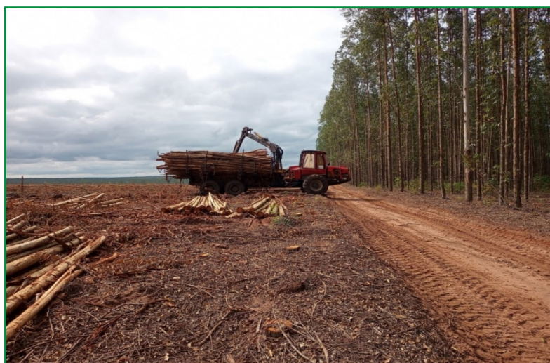
Figure 2 – Extraction machine adopted in the forest company (Forwarder)
