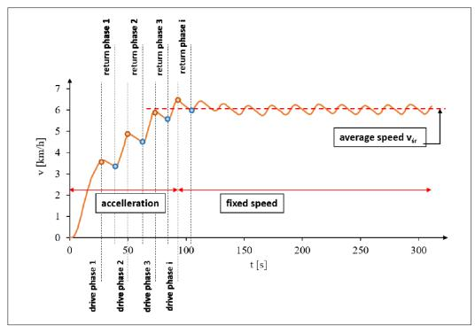
Figure 4 – Change of speed over time during wheelchair propulsion
