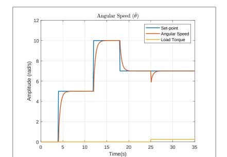
Figure 11 - Closed-loop system behavior for an input torque load
