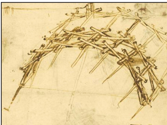
Figure 1 – Da Vinci's drawing the self-supporting bridge
