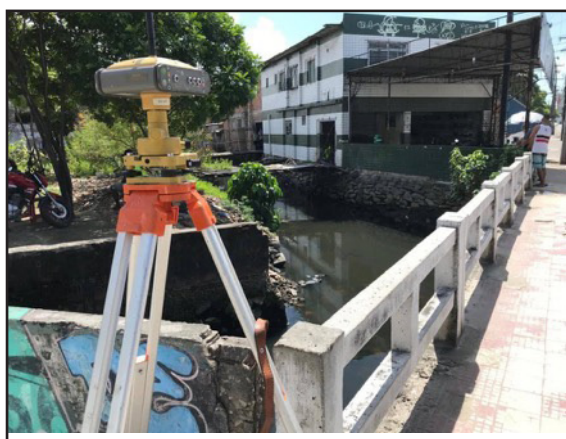
(a) Survey of orthometric altitudes and geometric leveling of the monitoring point
