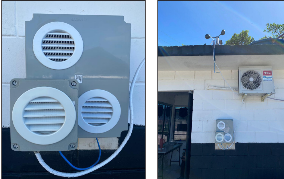
Figure 2 – Images of the project's meteorological station prototype installed on the field (wall facing South)
