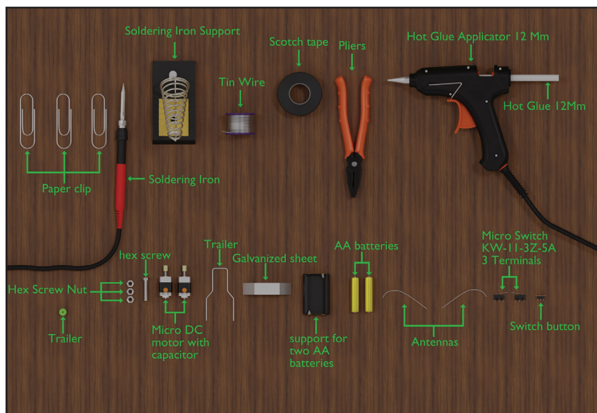
Figure 2 – Materials used to build the Robot
