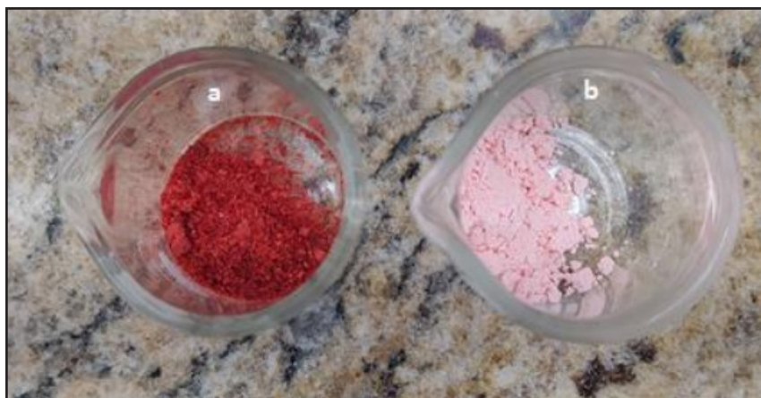
Figure 1 – Acerola powder concentrates (a) with freeze-drying and (b) with spray dryer
