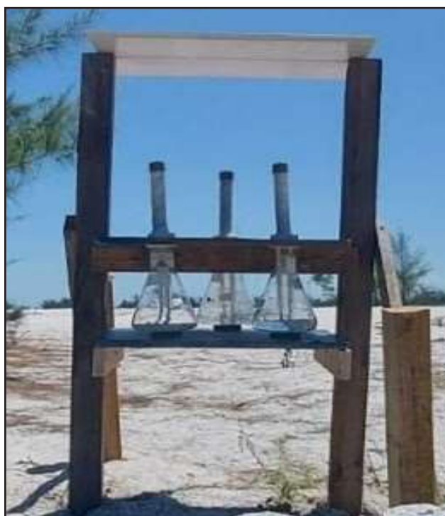
Figure 3 – Wet candle exposure station
