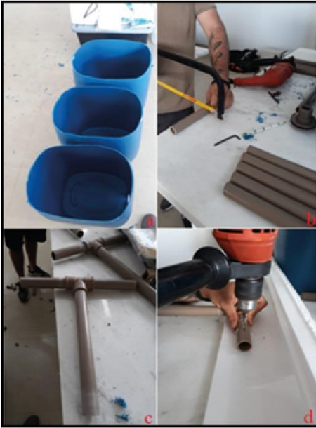
Figure 4 – a) Section of the cylinder cover; b) PVC pipe cutting; c) T-connection of the pipe; 5 cm spacing holes in the pipe
