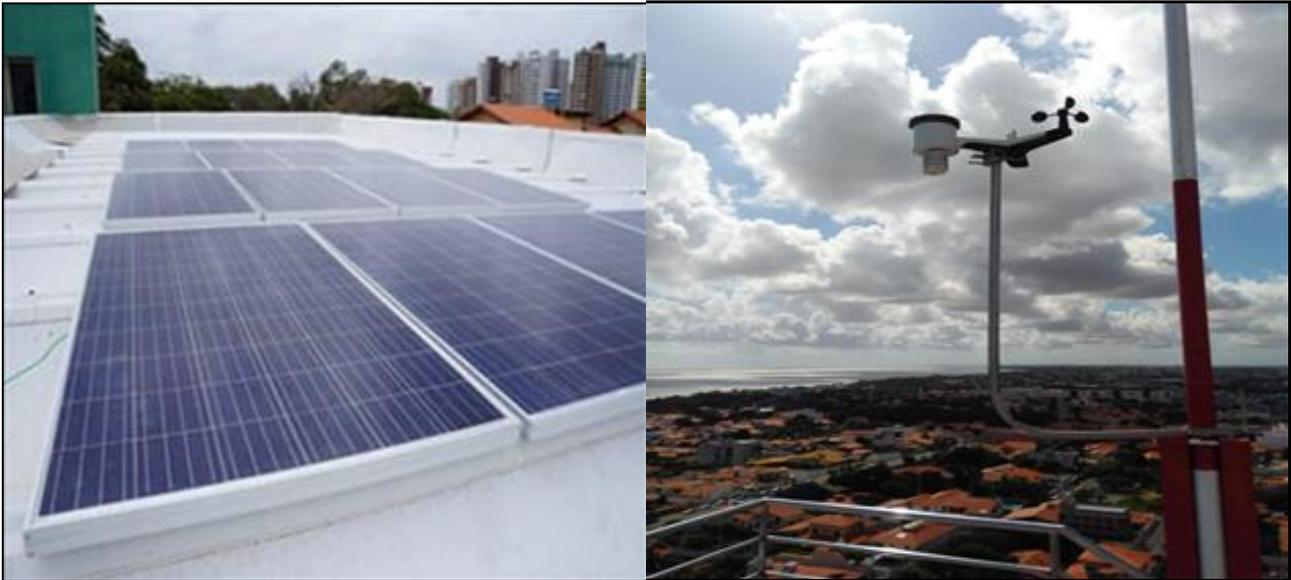
The operating temperature of the PV cells is a key variable for the energy production, strongly influenced by weather conditions. In this work, the operating temperature was estimated by integration of the meteorological variables related to wind speed ( $V_f$ ), ambient temperature ( $T_a$ ), global irradiance ( $G_T$ ), and mounting coefficient ( $\omega$ ) (SKOPLAKI *et al.*, 2008) — see Equation 1.
